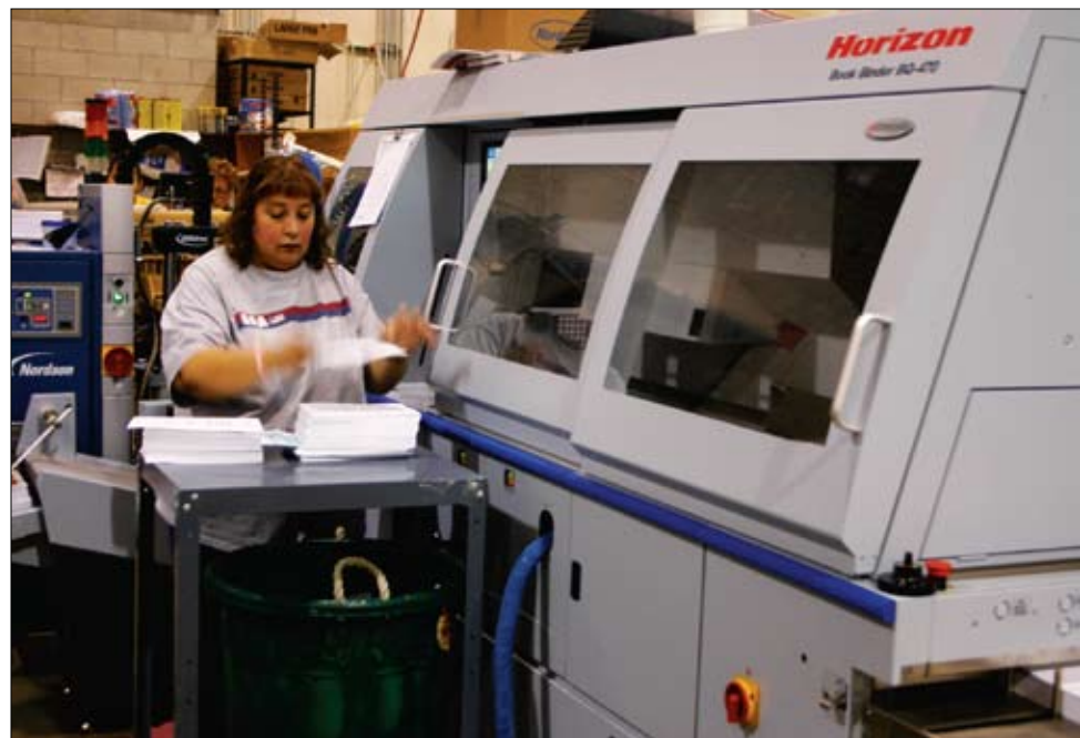
An operator at Publishers' Graphics keeps pace with a Standard Horizon BQ-470PUR perfect binder, which produces lay-flat books.
