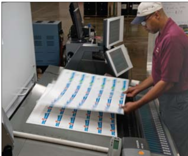
A printed sheet coming off the Komori LSX8402RP press is inspected for color by a worker.
