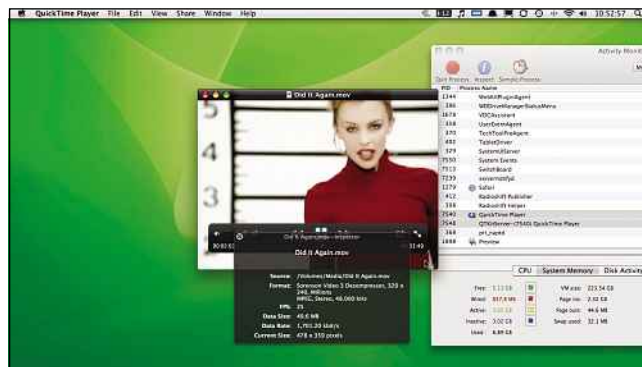
◀ This file is encoded using the Sorenson Video 3 codec, once popular for trailers and enhanced CDs. QuickTime X is using QuickTime 7 to play it, indicated by the QTKitServer process in Activity Monitor.
