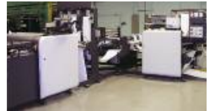
Flex Book bolts onto the HP T300 and keeps up with the press to produce book blocks
